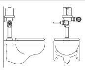
HYBRIDFLUSH® shown on water closet (toilet) with mechanical flush handle.
