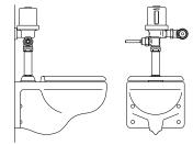
HYBRIDFLUSH® shown on water closet (toilet) with mechanical flush handle
