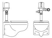
HYBRIDFLUSH® shown on water closet (toilet) with mechanical push button.
