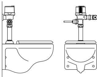
HYBRIDFLUSH<sup>®</sup> shown on water closet (toilet) with manual flush handle.
