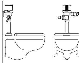
HYBRIDFLUSH<sup>®</sup> shown on water closet (toilet) with manual flush button.
